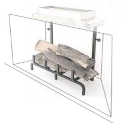
Visibly inspect that the **HearthCAT™** hood is flush against the back wall of the fireplace. If there is a gap of more than 1/2", then the smoke deflector must be installed in the back of the hood. Refer to the *"Installation of the Smoke Deflector"*.
