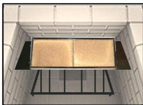
If the fireplace has a back wall width less than 26”, the **HearthCAT™** hood should be installed with the short side against the back wall (as shown on left). If the back wall width is greater than 26”, the long side should face the back wall (as shown on right).
